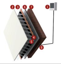
Confirm parameters of the electrical wiring system, ensure that a demand for electric power is sufficient. If the parameters are not sufficient, you should increase their values. Check humidity of the base floor. If it exceeds by 2%, use damp proof insulation.
