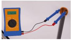
Make a subsequent measurement of a resistance using an ohmmeter. Draw a diagram a position of each strips electric wiring and temperature sensor.
